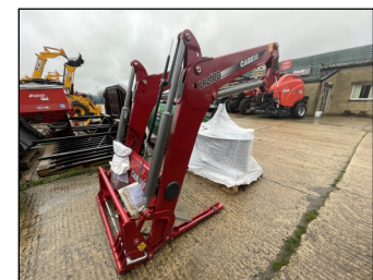
New Case IH LRZ100, Parallel lift, 3rd service, 3.85m High, 1860kg lift, euro 8 headstock. £POA
